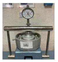
Figure 3: Testing of quasi-soil samples on a uniaxial compression apparatus.
